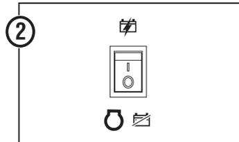
**NOTE:** This unit has a **GASOLINE OFF** setting that can be used before storing the unit for long periods of time. Refer to the user manual for details.
